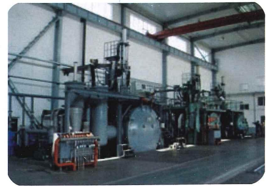
© Vacuum smelting casting equipment , Function: Smelt and cast the parts of titanium, zirconium and its alloys 800kg Vacuum consumable electrode condensing fumace:1 set 500kg Vacuum consumable electrode condensing fumace:2 set
